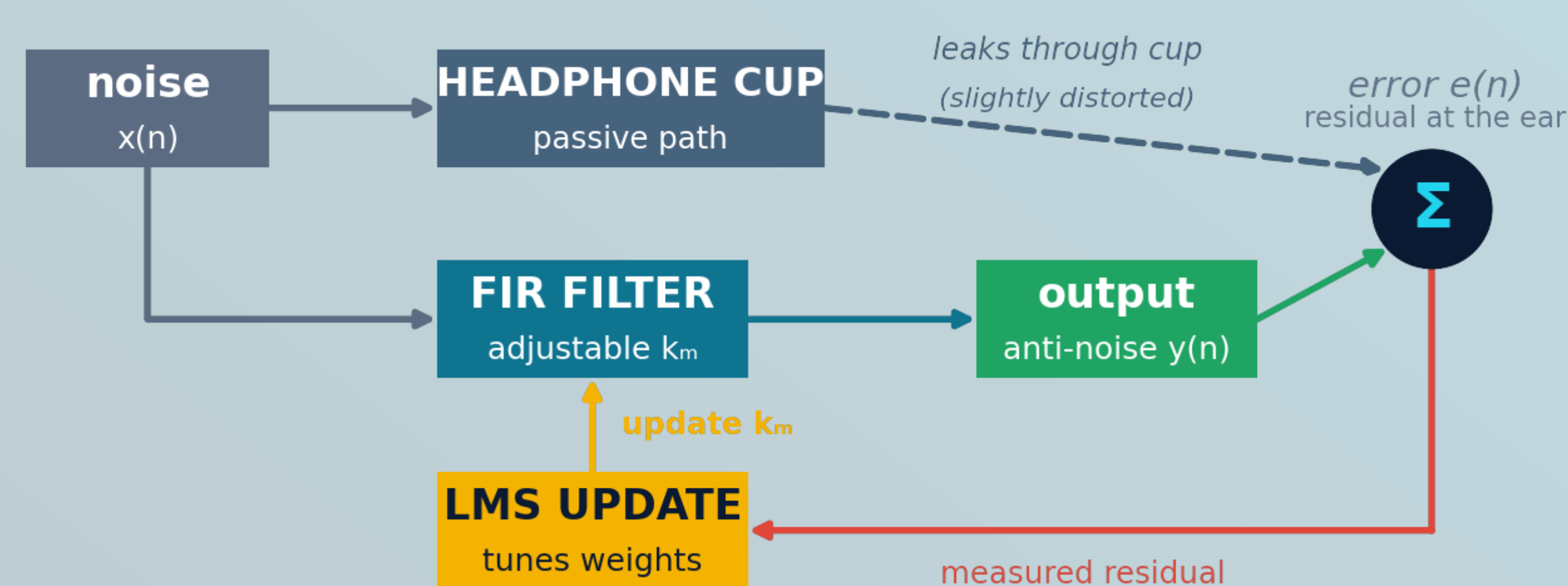
System architecture: passive cup path, adaptive FIR, and the LMS update loop
