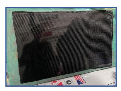
Above: Carbon Fiber Skins (four ply) resin infusion setup and finish
