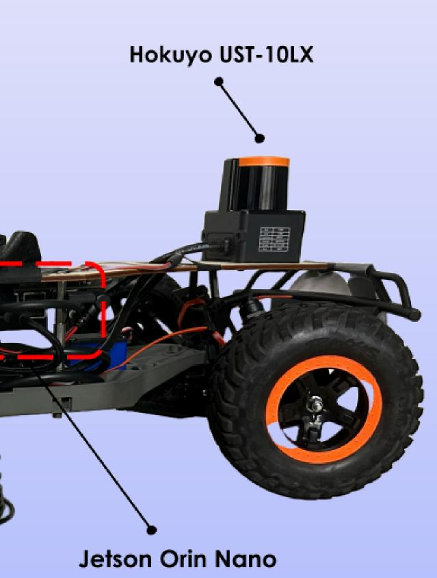
2D LiDAR with high-speed and accurate measurement data with its 40 Hz sampling rate in a 270° field-of-view up to 10
