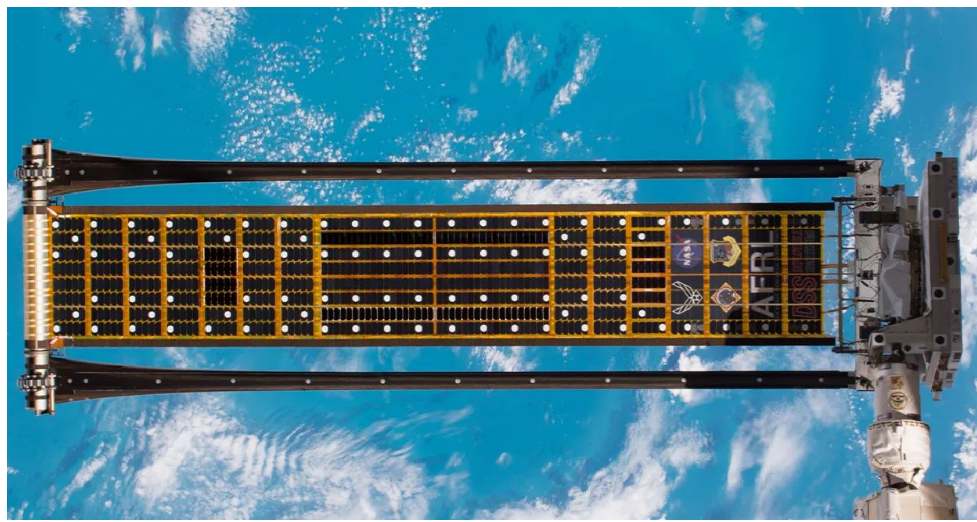
Figure 1: Image of the ROSA being deployed on the ISS.
