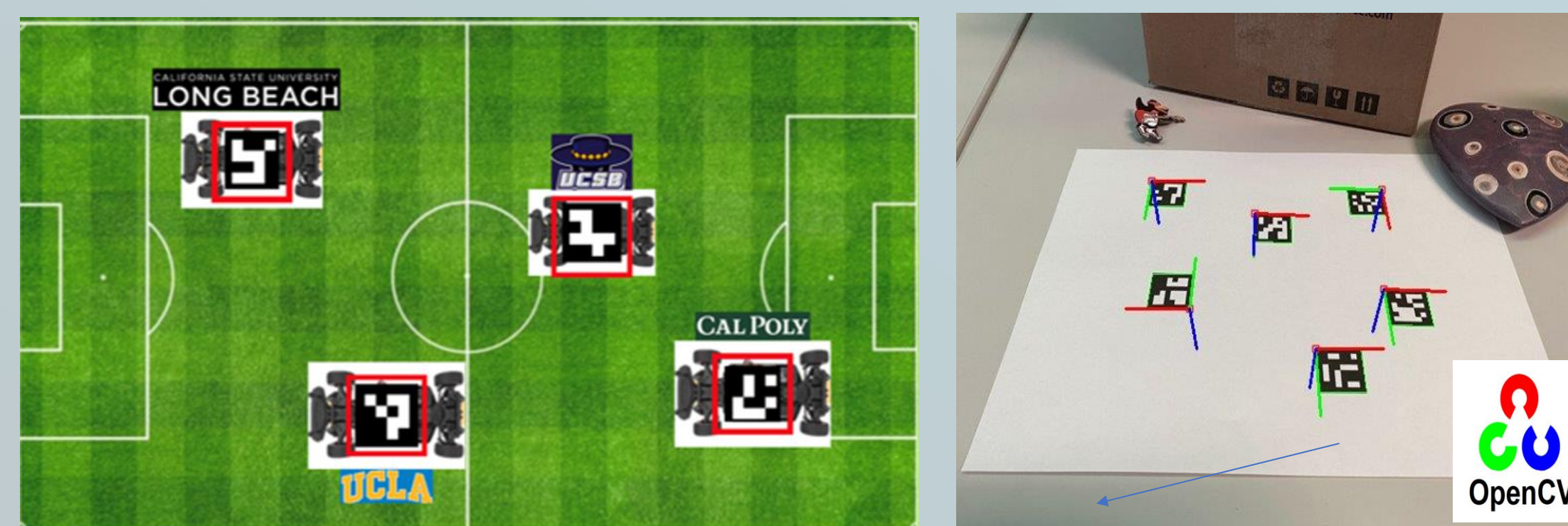
Figure 4: ArUco markers and pose estimation.
