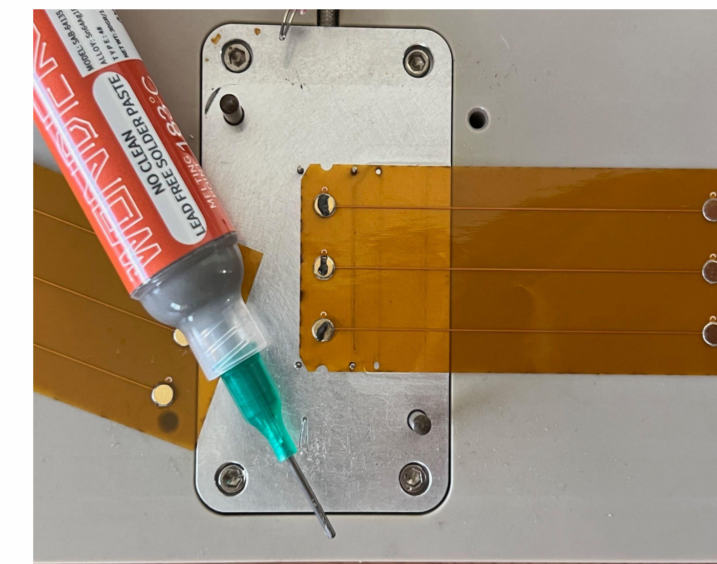
The left image shows solder on the flex PCB's pads, and the right image shows a successful connection.
