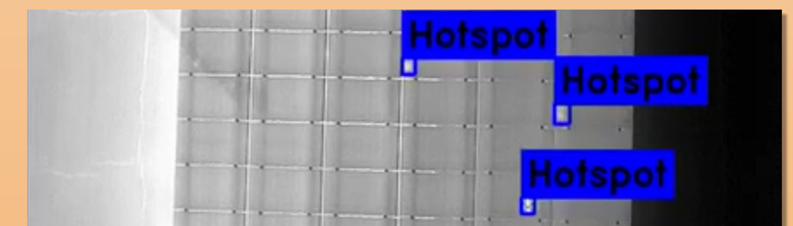
Simulated output of live filtering on IR finding hotspots
