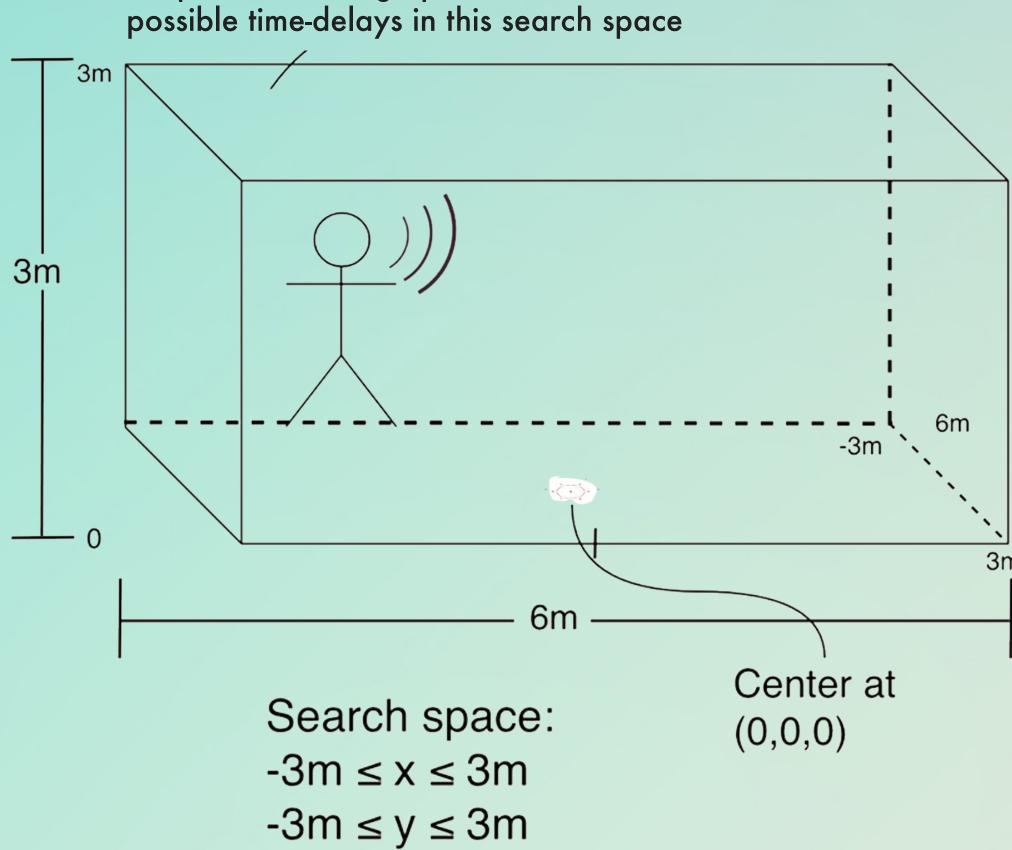
The phase-matching optimization procedure is similar to doing a least-squares fit. To do the phase-matching optimization, we compute the Circular Integrated Cross Spectrum (CICS) of the sound received by the microphones.
