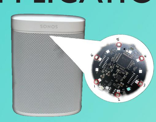
The microphone array lies flat inside the SONOS One speaker, and is used for voice command features. Our position estimator can be incorporated into the SONOS One without hardware changes.
