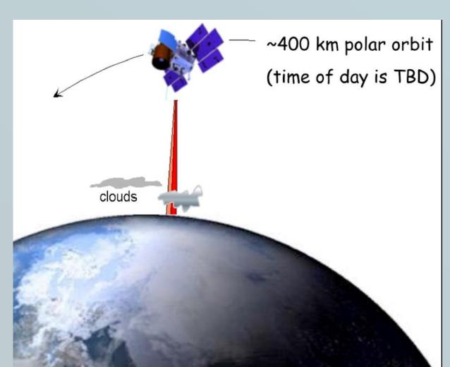
The IMPRESS Lidar system is designed to measure the concentration of atmospheric CO<sub>2</sub>. Small enough to fit on a satellite, it includes a master and slave laser integrated on a single photonic integrated circuit (PIC) along with associated electronics. The master
