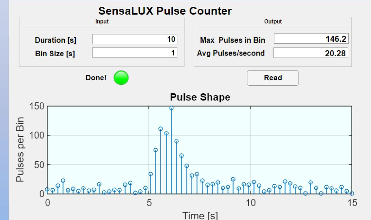
This image displays the user interface of the  $\mu PMT$  based design during a simulated bioluminescent reaction. This user interface plots the transient response of the luminescent reaction, as well as providing important statistics about the light entering the system.
