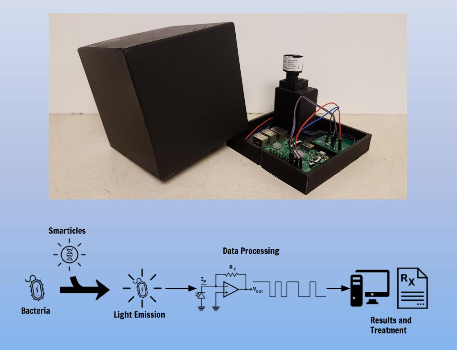
The system we created can very accurately measure low levels of light emitted from a bioluminescent reaction. By analyzing these measurements over time, bacterial antibiotic resistance and vulnerability can be determined quickly and cheaply.
