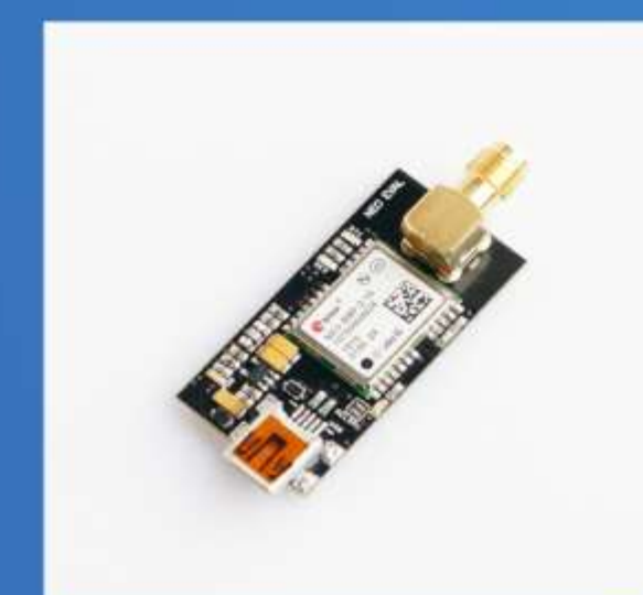
GPS Gives position of pod along I-beam in real time
