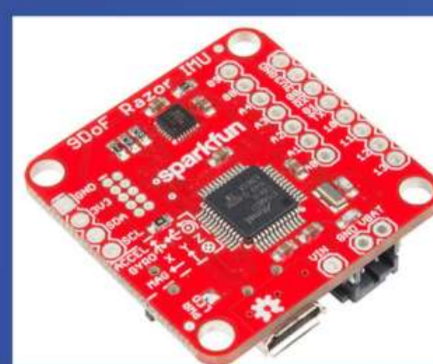
IMU Gives acceleration and rotation of pod in all 3 axes
