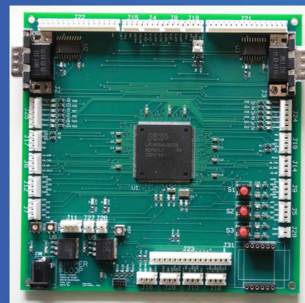
PCB Primary control unit and sensor monitoring system
