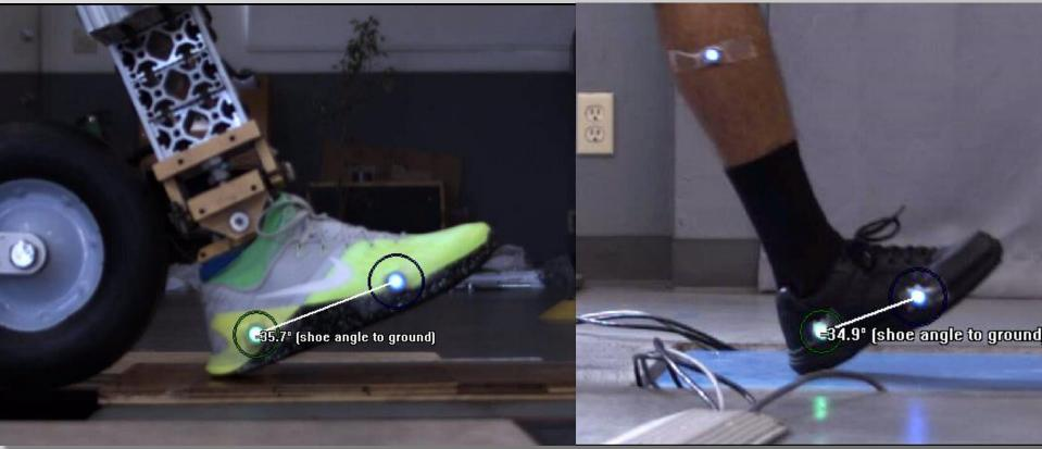
Figure 4: Motion tracking comparison for TRAX and human
