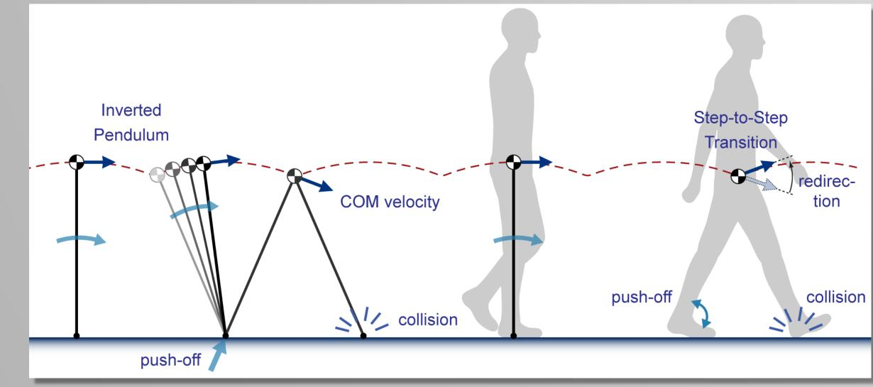
Figure 1: Inverted pendulum model for human gait
