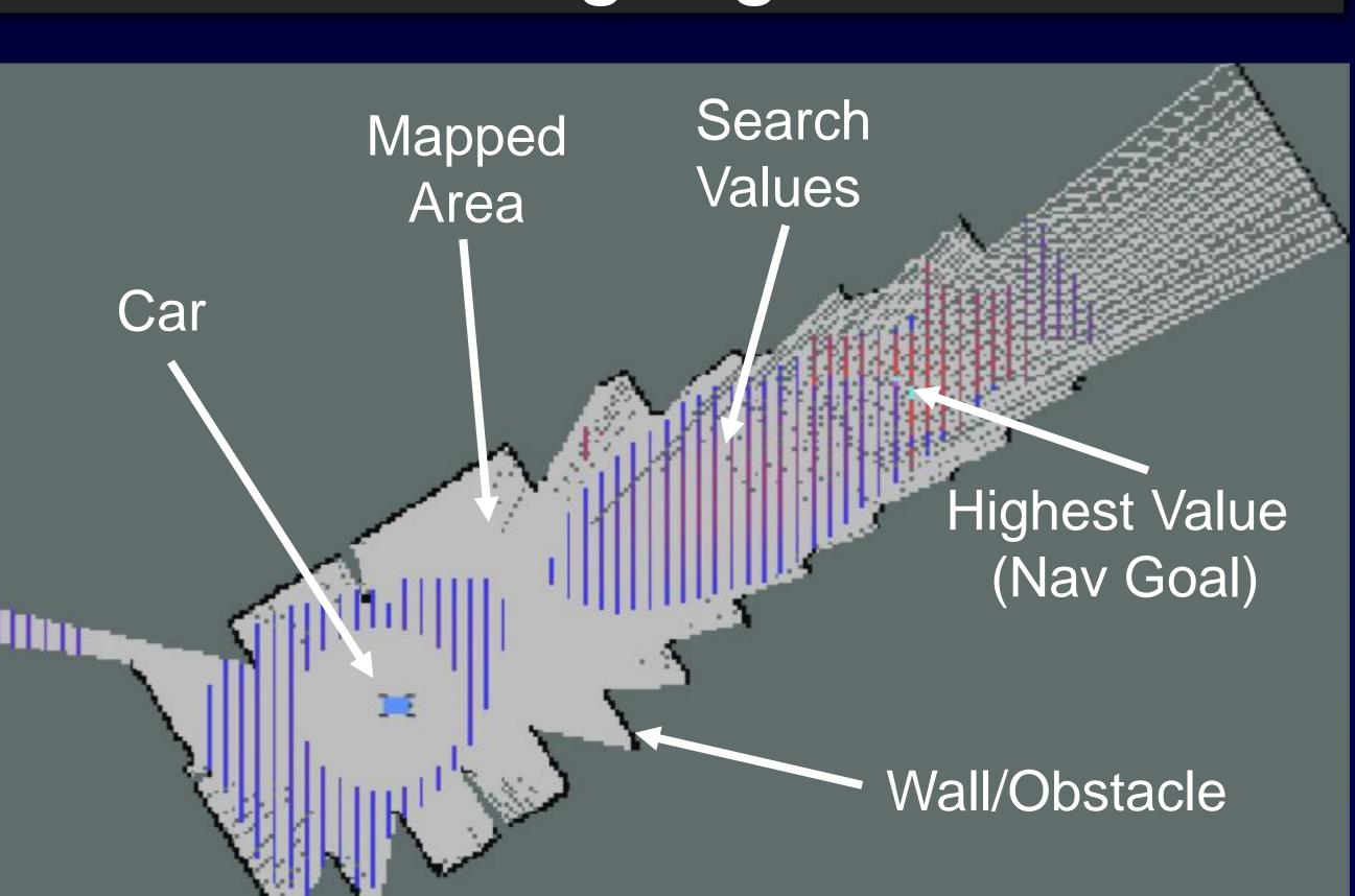
The Searching Algorithm uses the SLAM map and assigns values to points based on aspects such as unsearched areas, obstacle locations, ease of travel, unmapped areas, and time since a point was last seen. These values are shown as the colored stripes with red being a higher value. Velma then constantly navigates to the high value points until the target bucket is found and reached by the vehicle.
