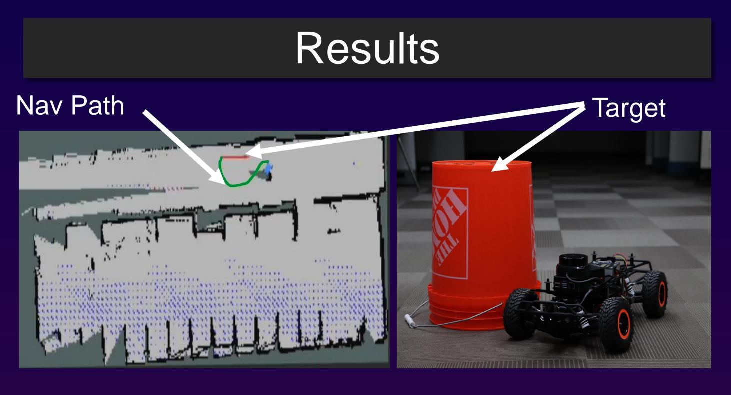
Velma was able to find the target bucket in multiple configurations of various difficulties in under three minutes. Potential improvements include faster map updates, improved path planning algorithm, and add LEDs for headlights, brake lights, and status indication.
