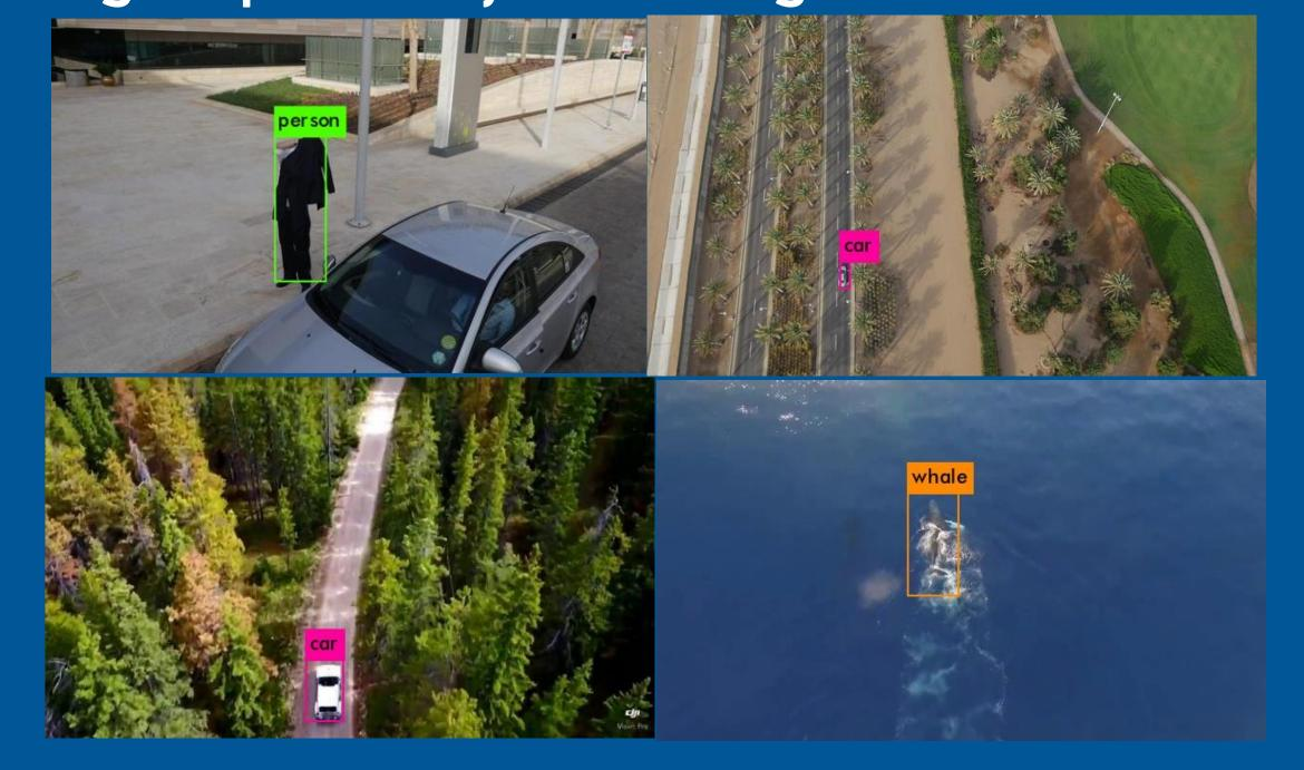
In real time detection, CNN (Convolutional Neural Network) uses the weights trained from the previous dataset to infer objects in each frame of the video. This is done through many convolutional layers with different resizing schemes. The CNN network divides the image into regions and predicts bounding boxes and probabilities for each region.
